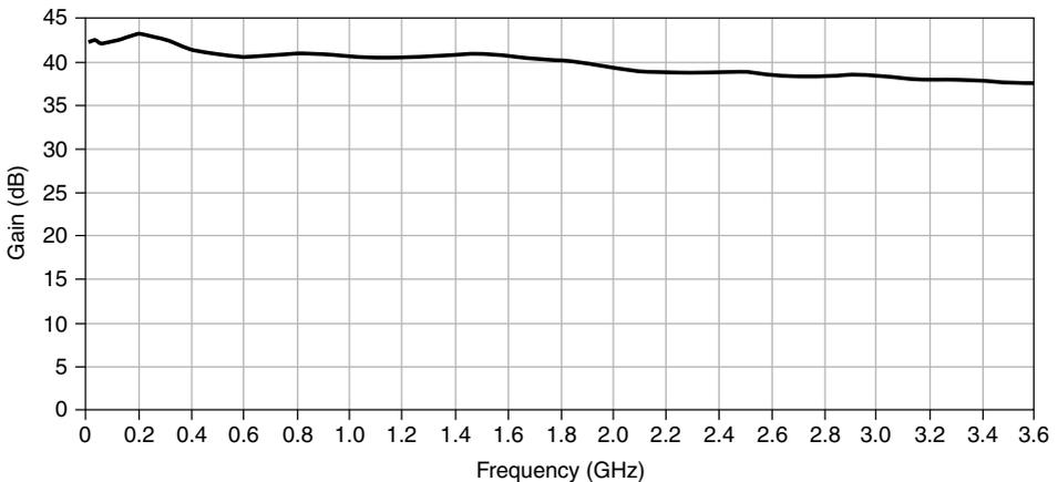
**Figure 17.** PXle-5605 Typical Low Band Conversion Gain (Center Frequency <3.6 GHz)
